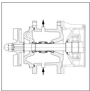
Fig. 6: System with sealing pressure (SK)
