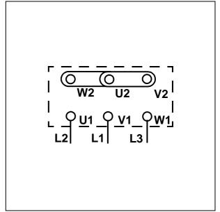
Fig. 3: Connection diagram for three-phase motors, circuit Y
