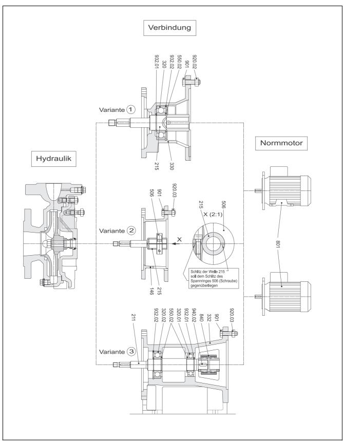
Fig. 17: Shaft assembly of bearing pedestal
