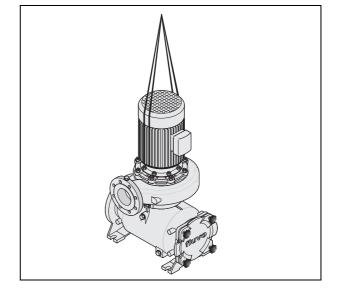
Fig. 1: Example of slinging for lifting
