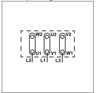
Fig. 2: Connection diagram for three-phase motors, circuit  $\Delta$
