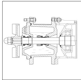
Fig. 7: System without sealing pressure (TLS) GLRD "Tandem"
