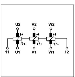
Fig. 4: Temperature sensor built into the bracket head and insulated. (Max. permissible voltage 2.5 V per sensor)
