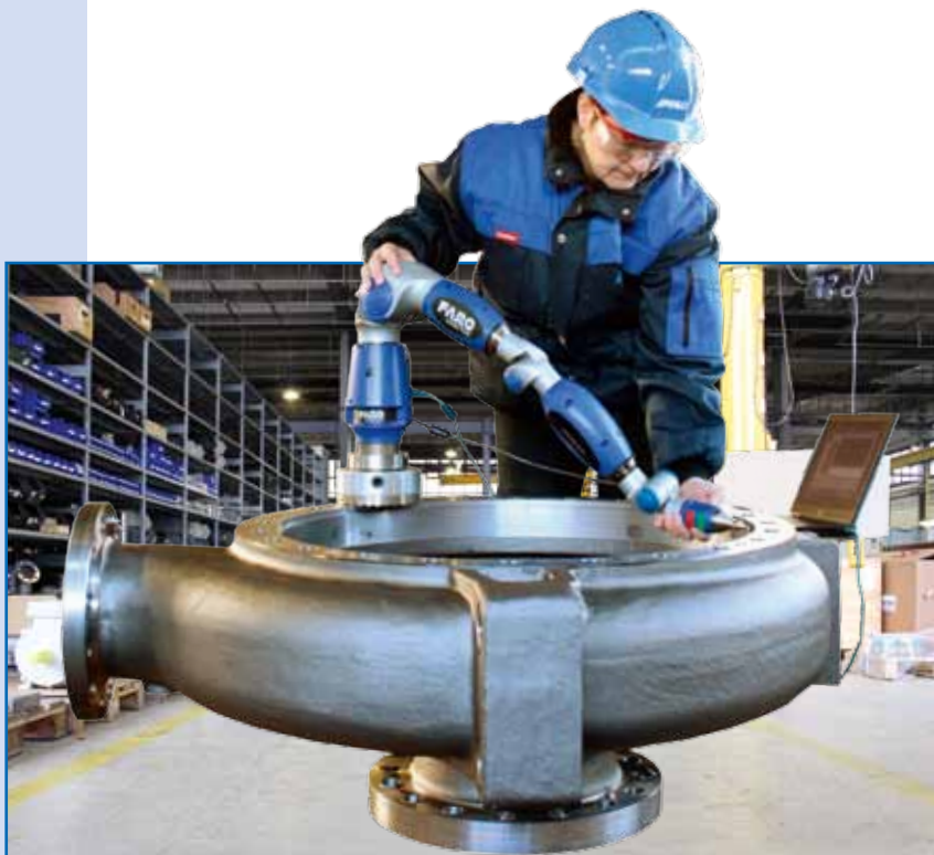
■ Quality Assurance also in local application by means of flexible portable 3D-Coordinates Measuring Unit.
