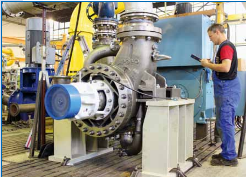
■ Heavy-duty APOLLO-process pump with two-stage according to API for Offshore application on the test field.
