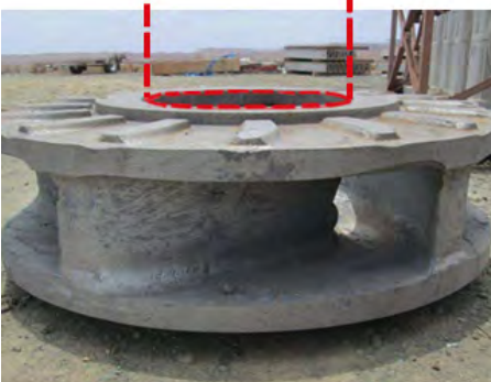
millMAX pump impeller eye protected from recirculation wear by the wear ring.
