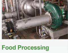
Impeller design has a large eye area for low NPSHr and increased vapor-handling capability with higher performance. Ideal for food handling, hot cooking oil, blanching, waste handling and wash-down.
